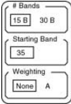
To choose the number of bands displayed, the starting band and the weighting function, use the **FREQ** menu. The **FREQ** menu will display the band selection menu shown at the right whenever octave analysis is on.
