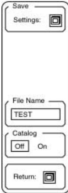
**Save Settings** Pressing this key will save the current analyzer settings to the file specified in the File Name field.
