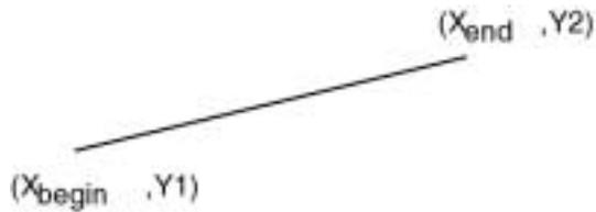
A segment may be defined as either an upper or lower limit. Trace data values which are greater than an upper or less than a lower limit cause the test to fail.
