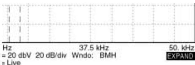
The **Top reference** is the Y value of the upper edge of the graph. The units can be Volts, dBVolts, or EU (user defined engineering units). The **Vertical** scale is shown as the number of dB, Volts, or EU per division. This value is changed whenever the vertical scale is adjusted.
