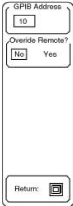
**GPIB Address** This key activates the GPIB Address entry field for numeric and knob entry. The instrument address can be set from 0 to 30.
