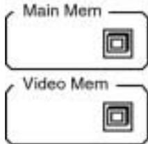
**Main Memory** Pressing this key tests the program ROM and data RAM on the CPU board. The data acquisition memory is not tested. See the Test and Calibration section for more information on testing the data acquisition hardware.
