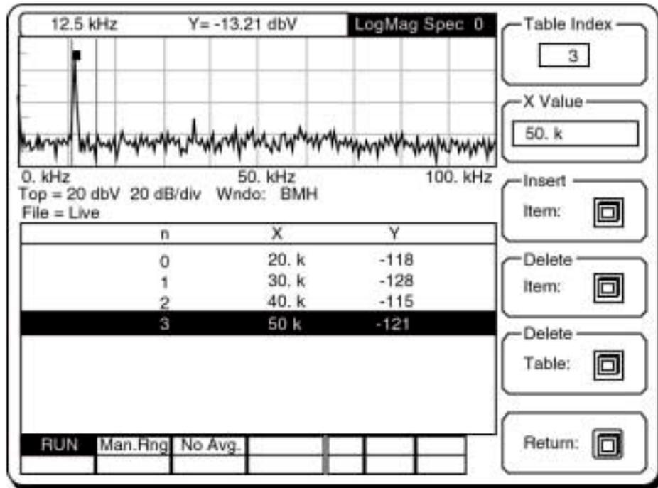
A sample data table display is shown above. The table entries are n (table index or line number), X (user defined X values), and Y (measured data values corresponding to the X values). The Y value is actually for the frequency bin which is closest to the entered X value (within one bin resolution). The Y values shown in the table are in the units of the display. X values which are not in the frequency span have the message OVRG for their Y values.
