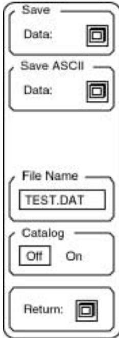
**Save Data** Pressing this key will save the active trace data and associated parameters to the file specified in the File Name field.
