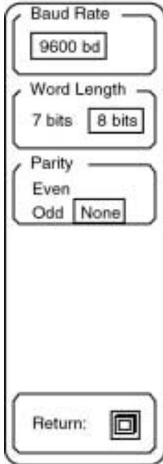
**Baud Rate** The Baud Rate key allows the knob to adjust the RS232 baud rate. The baud rate can be set to any standard value from 300 to 19200 baud.
