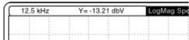
Any previously highlighted parameter field will become non-highlighted. Pressing a soft key to highlight a new parameter field will let the knob adjust the new parameter while the marker becomes unselected.
