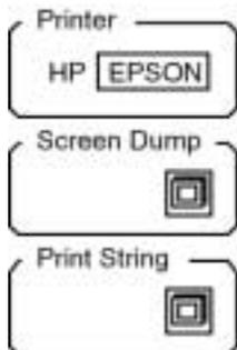
**Printer Type** The Printer Type key selects the type of printer attached to the parallel printer port. Any Epson compatible graphics printer or HP LaserJet compatible printer is supported.
