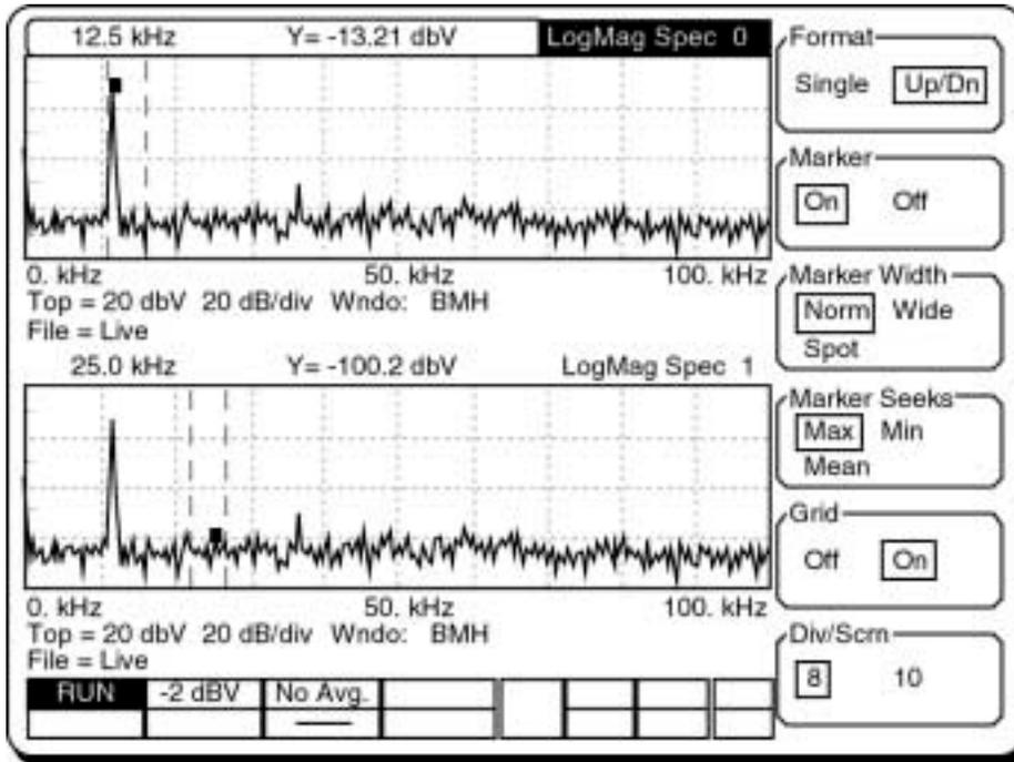
The dual trace or Up/Dn format is shown above. The display format is selected in the DISPLAY menu. Trace0 is always the upper trace. Each trace is annotated the same way as the single trace.
