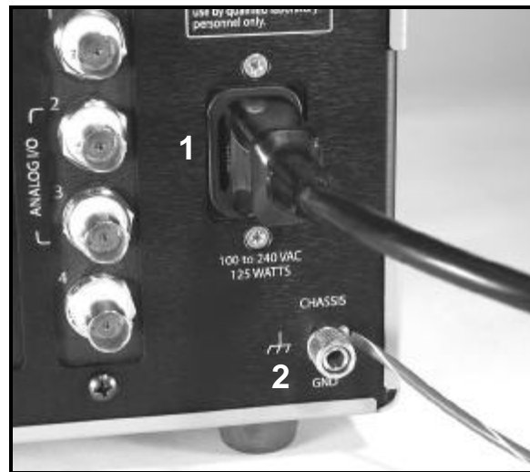
Figure 1-2. Power and chassis-ground connection on the back of the PPM100 controller. 1. Power entry module with power cord (connected to grounded wall outlet on the other end), 2. CHASSIS GND lug with heavy gauge ground wire connected directly to facility earth ground.
